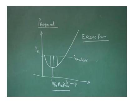
Now, if you again revisit power required versus speed or velocity, graph is also looks like this. And let us say, this is the power available, typically, a proper layer I C engine combination, where the power available almost remain constant for practical purpose, as far as understanding the basic physics behind it. In actual practice, please remember, there are secondary effects, we will be talking later.
