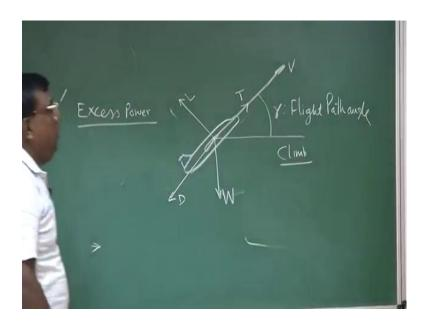
Let us draw this diagram, this is a typical schematic representation of an airplane, which is not cursing, it is now climbing, you say it is climbing or flight phrase is climb. Let us see here, if I now try to write the force balance along the velocity direction, along this direction, what do I get? I get of course, there is a thrust.
