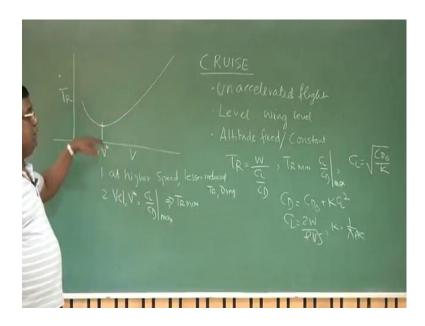
Yes, welcome back to this additional session. Let us revised, what we have covered so far, we were focusing on cruise flight. And what do you understand by cruise flight, cruise is, it is an accelerated flight. Number 1; un accelerated flight and when you say level cruise, level means wings level; that typically it is like this. If I am doing a cruise, I am going the constant speed, wings level not like this, wings level like this and also I am ensuring that, there is no change in the altitude.
