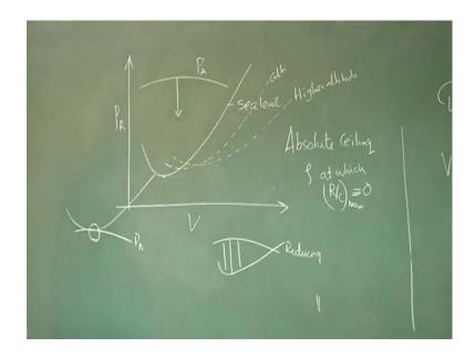
So, the power required suppose this was C Level as I write C Level condition, I can see from there, as I am going to fly at a higher altitude keeping same C L, the velocity which was here, now I require higher velocity. So, you will find the graph, this is altitude, then further, this is higher altitude. What happens to thrust or power available, the power available let us say here, typically for I C engine, popular combination.
