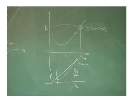
We also realize that, this power required verses V, if I draw like this and if this is typically for a I C Driven popular combination engine, this is the V max and for jet engine, if you want to draw it like this. Again, this is the power required, the jet engine, this is the power available; this is for jet engine to see this point is the V max. But, as a designer, we need to also that if I am coming for a landing, I will be operating somewhere here. So, I have got enough excess power.
