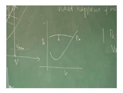
So, this is important, because please understand, we are writing power required verses V plotting it like this, this is friction altitude. As I am going higher and higher, the density of air is reducing, so that, will have an effect on this. Second thing for evaluable again as we going higher and higher density is going to reduce. So, this also will have an effect on
