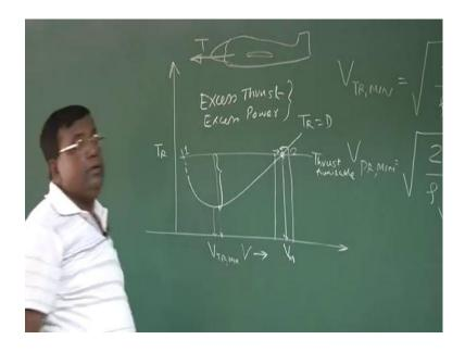
Now, let us see, we have also seen this thrust required versus speed or velocity, the graph typically goes like this and this is the point, where the V for thrust required minimum. Please remember, thrust required is equal to drag. So, when I say thrust requirement minimum, I am implicitly say this is telling that, the drag required minimum. Now, come back to the engine, the airplane has an engine, it will be delivering some thrust.
