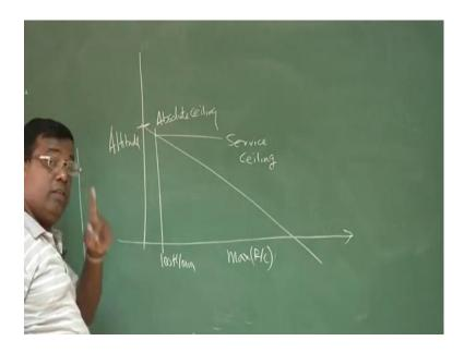
So, how it is generated, if I draw a graph, this is altitude variation can be and this is maximum rate of climb, graph is something like this, here this altitude is called absolute sealing and we for practical propose. We define an altitude, which is called service ceiling is called service ceiling is an altitude at which the maximum rate of climb is not 0. By it is 100 fit per minute for all operation propose, we use service ceiling not absolute ceiling.
