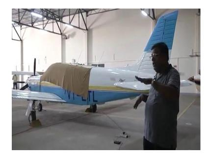
Also, you could see that these are the landing gear, and they are not retractable type. We have Piper Saratoga where the landing gear goes in. So, once it is flying in air, landing gear is out, then that offers resistance. So, that is and now what you will find for such airplane. But, for bigger airplane or even for Saratoga what happens; the moment I take off, the landing gear goes in, so the drag part is reduced.
