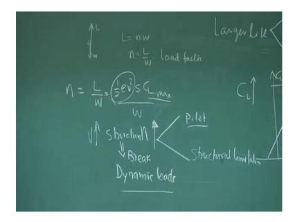
Since, I know n equal to lift by W and n is nothing but, half rho v square S C L by W. Let us say, I am flying at C L max, because I know beyond this C L max I cannot fly, because I will be going into a danger zone, which is a stall for us. So, I am fixing that C L max, but I argue I will still increase this n as I go on increasing the speed.
