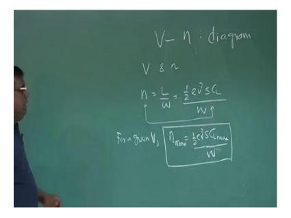
So, that is exactly is called V n diagram, that is typically V n diagram represents or for a pilot, when he sees a V n diagram he knows what are the speeds he should avoid, what is that envelop, he should know a priori, because he go for flight.
