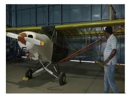
We were showing tricycle type landing gear, but if say this is an airplane, this Piper Super Cub, one of the very powerful airplane we have been using it for long, for more than 40 years. Now, this is grounded and we are using it for static demonstration. You could see here, this is not a tricycle type landing gear. This is basically a tail dragger, there is a tail wheel landing gear there and two here. What is the difference between this configuration and the tricycle configuration?
