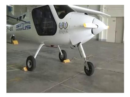
Please draw your attention to this part, which is the landing gear and you could see, this type of configurations are called tricycle landing gear, one nose wheel and two rear wheels. When we are going for a takeoff ((Refer Time: 00:52)), at an appropriate speed the nose will be just high like this and it will continue and lift off and then, it will do like this for a cruise.
