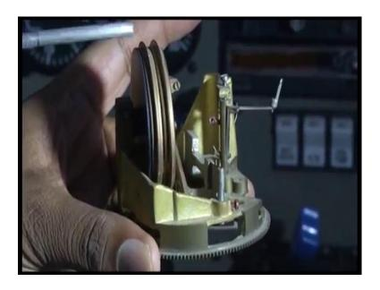
This is an instrument inside, this is a specially treated metallic corrugated diaphragm made of nickel silver or phosphor bronze, which is fitted inside the case on a frame. You can see that, it is fitted on a frame.
