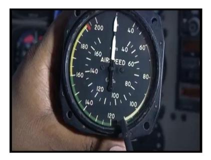
So, you can see this is the airspeed indicator; there are various coloured markings in this airspeed indicator. First of all you can see the red line, which is the maximum speed or it is the never exceed speed, we call it VNE. The airplane should not be operated beyond this speed. Then, you can see the yellow markings, from here to here you can see the yellow markings. This is the caution range, in which the airplane has to be operated with caution in smooth air conditions only.
