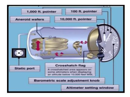
The altimeter is connected through the tubing to static vents, the static pressure through the static vents and the tubing enters the static port.
