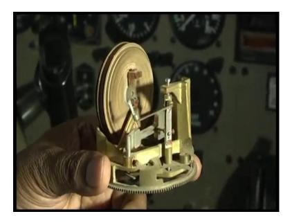
This diaphragm is connected to the pitot pressure, the pitot pressure enters the diaphragm from this hole.
