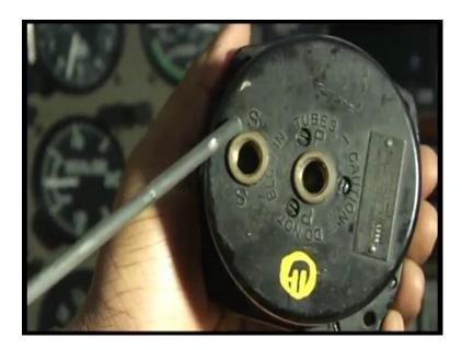
It consists of an air tight case. At the back of with, there are two connections one for static pressure. You can see, this is the opening for the static pressure and the other for the pitot pressure, you can see S written and P written here.
