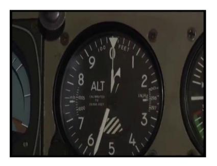
So, now we will talk about altimeter, this is the altimeter on the instrument panel. The altimeter works on the aneroid barometer principle, which is calibrated to read height. The altimeter is used to give a continuous indication of height on an aeroplane above any reference point.
