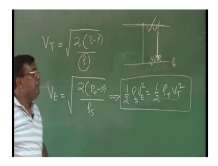
So, this V is basically true airspeed, because rho is the actual density at the altitude you are flying. But, for calibration purpose you could understand, every altitude getting density and all, then calibration will be a difficult thing. So, we have defined some speed V E, where this is same dynamic pressure; however, rho is rho S which is the sea level standard atmosphere value. Now, if I again see this expression little carefully, what does this expression means to us?
