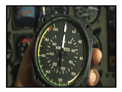
It is basically a differential pressure gauge, which measures the difference between the static pressure and the pitot pressure. The static pressure is the pressure of the atmosphere around the aircraft, the pitot pressure is the impact pressure what develops in the pitot pressure tube due to the motion of the aircraft.
