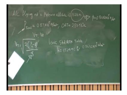
Let us say one aircraft, which is flying at a pressure altitude of 1524 metre. The aircraft flying at a pressure altitude of 1524 metre and P total, let us say the aircraft measured was 0.87 into 10 to the power 5 Newton per metre square. Please understand, this is the P total that is a central tube of the pitot's tube. Let say, it was measured to be 0.87 into 10 to the power 5 Newton per metre square, calculate V true and V equivalent.
