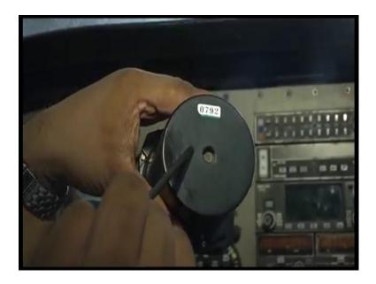
The altimeter at the back has got one port only through which the static pressure enters. This instrument is inside the casing; the static pressure enters through that port and acts over this capsule. When the airplane climbs, the atmospheric pressure inside the case that is outside the capsule decreases, this causes expansion of the capsule. This movement of the capsule is transmitted to the arm, magnifying lever, sector, pointer pinion and pointer.
