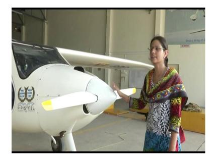
This is Sinus 912 aircraft which is a motor glider and its manufacturer is Pipistrel. So, we will today we will discuss about the structure and the instrument panel of this motor glider. This is an all made its construction is of composite material. This is the spinner of the aircraft having a 2 bladed propeller which is vireo. Then, it has a rotex 912 engine installed in it which is a 4 cylinder engine and it is a piston engine 4 stroke.
