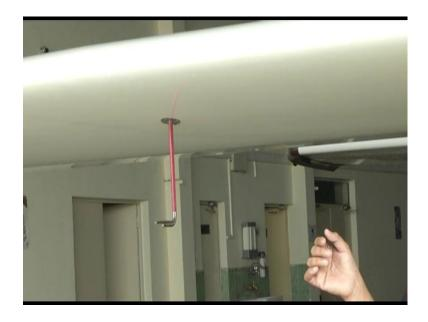
Then, it has a wing span of 15 meters. For this wing contains a flaperon. Normally all aircrafts have either aileron and a flap, but in this varying motor glider the 2 control surfaces are combined in one and then that is of flaperon which consist of a flap and aileron that helps in rolling and as well as at the time of takeoff and landing.
