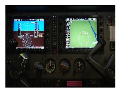
As far as of now we have learnt about the conventional gauges that was been introduced in the earlier aircrafts, but nowadays the modern cockpit is being introduced that gives a display, a screen and a display on that screen inside the cockpit. Earlier we used to have gauges like we have in this aircraft that is airspeed indicator, the instrument and the alternator.
