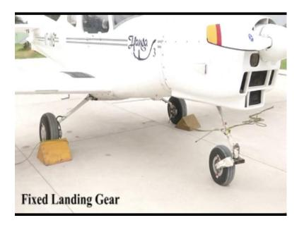
As of now we have studied about the aircraft structure and aircraft engine. Today we are going to see about something about the landing gears that is used to balance aircraft on the ground. And, so, we have 2 types of landing gears - one is fixed and one is retractable. Fixed type of undercarriage is this which you can see; this does not have a retracting mechanisms. This is the short strut on which the landing gear is balanced. This is the nose wheel; the inner 2 are the main wheels.
