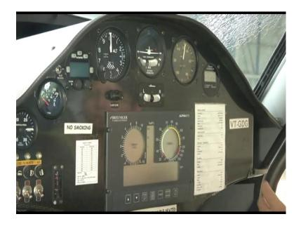
Now, we will move inside the cockpit to just have a brief view of the instrument panel and the controls. So, this is the instrument panel of the motor glider which we were discussing about just a few minutes back about the composite motor glider sinus 912. This complete is the instrument panel which consists of an alpha m f t installed in this center which gives us the readings of various engine instruments; and, apart from that various airframe gauges.
