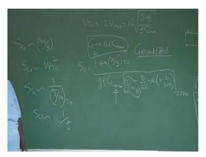
What do I see? I see S G is proportional to W by S that is, if reloading is less S G is less. Wing loading is less means large wing, but the probably with large wing is large wing mean large drag, so there is a conflict. So, designer has to see what, how do I handle this and you will see that, that is why high speed airplane they do not want very high span wings, they are low span wings, low aspect ratio wings by now you understand.
