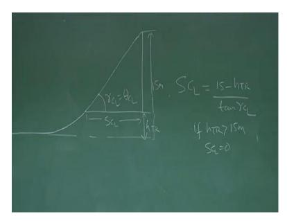
Finally, we are left with which is gamma C L many book will I theta, theta C L and find out this distance which is S C L and you know there was the pull up, where the role and like this and let say this distance is from the ground, let the distance the h T R. So, I get easily find out S C L by using this relation S C L equal to 15 minus h T R by tan gamma C L if h T R greater than 15 meter then S C L equal to 0 this is by simply by this geometric.
