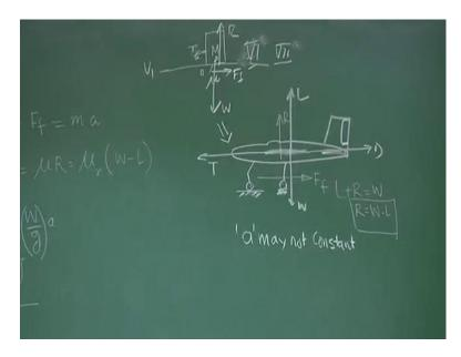
Now, what is happening here? Let us see this, what is happening here. So, let me first write the equation the way I wrote for that, this is T minus D minus because of the wing in contact with the surface, the landing gears. I say net frictional force is F f and let see the ground reaction is R and weight is W. So, one thing I know that here let me complete this L plus R equal to W or R equal to W minus L, naturally if lift is equal to weight then R will be 0, this I know.
