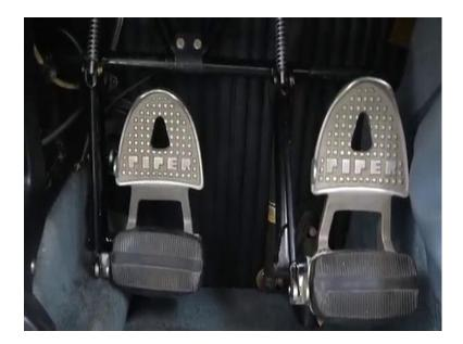
Now, I will turn the aircraft to left both the pedals are at the same level that is at the neutral position see the left pedal is moving inside the aircraft is moving is turning to left. The aircraft is turning to left, you can see that now the right rudder pedal is going
