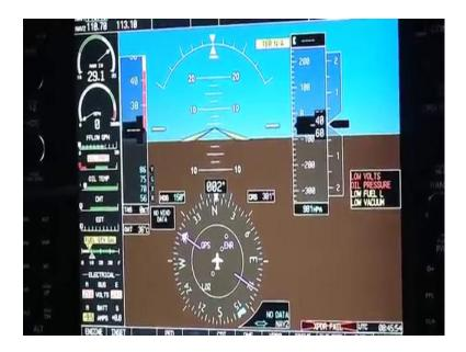
Now, we are sitting in modern cockpit, which is called also called a glass cockpit, this aircraft is Cessna 206 H, newly inducted in flight regulatory I I T Kanpur this aircraft has got carbon 1000 avionics. As you can see, there are two screens in the front this is the first screen called the P F D that is the primary functional display, this is the second screen which is called the M F D which we call as multifunctional display.
