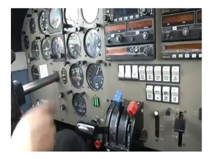
Then, we have the engine controls, this is the throttle control, the throttle the more the throttle you give the more the engine generates power. This is your propeller control with this, with the help of this control you can vary the blade angle of the propeller and this is your mixture control, with this control you can vary the mixture of fuel and air going inside the engine cylinders.
