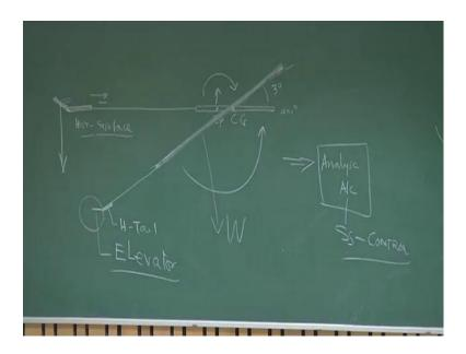
So, if you see here, this was the plate, this is the rod and here, I have put the horizontal surface to ensure that, the overall centre of pressure comes behind the centre of gravity. Although, please understand the moment I put a tail here, the original centre of gravity is supposed to come little backward. So, I am neglecting that, that is small, but more I am
