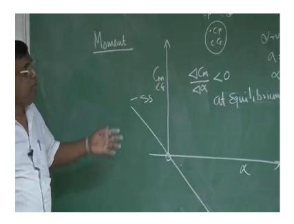
So, what we have learnt from this, whenever we are drawing C m, it is actually C m C G and alpha, whenever I am drawing graph like this, I should know that, it is about a particular C G. And for this plate or the aircraft to be statically stable, what is the condition, condition is the slope of C m versus alpha graph should be less than 0 at equilibrium, this is very important.
