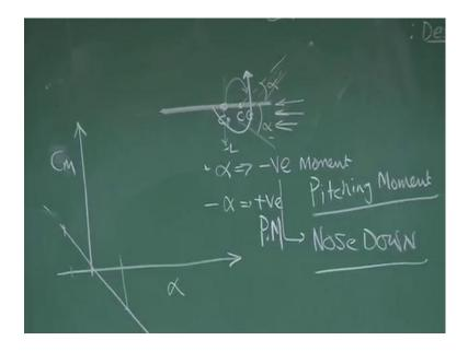
Again, we go back to George Cayley, suppose this is that magic plate and let us say center of pressure is here and C G is here. So, I am taking a simple case that, this plate is design such a way that you have given more mass towards the nose of this plate. So, that C G is in front of center of pressure or I say center of pressure is behind C G or center of pressure is at top C G and this is you know very well, this is statically stable case.
