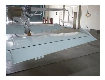
The most important part of an aircraft is the wing that is a lift producing device. The wing of Hansa 3 Aircraft is a single piece flying with front spar, the leading edge spar, main spar and the rear spa. It is of composite construction, because spars are around 10.5 meters consisting of a primary control surface. Aileron attached to a wing and a secondary control surface flap, which is located in both side of each wing.
