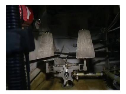
This is the controls tic, which is used to operate the primary flight controls, the aileron and the elevator. Moving it towards left or right gives the movement to the aileron and the rolling motion to the aircraft, moving it forward or aft gives the pitching moment to the aircraft, that is to the motion to the elevator and thus and aircraft pitching takes place.
