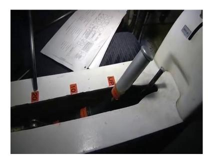
This the lever for flap, which has three positions after 10 degrees and 20 degrees after this flap fully up 10 degrees is, when flap is should crafted down wards to 10 degrees and 20 degrees, when flap is attracted fully towards down wards that is 20 degrees, 10 degrees is use of the time of takeoff to increase the surface area of the wing and to increased in the left, twenty degrees is used at the time of to increase more graft, another provides safe landing in a minimum distance.
