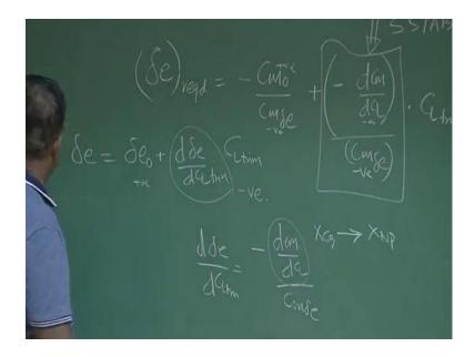
Now, how the slop will change, what is this slope, d delta e by d C L trim is minus d C M by d C L by C M delta e. So, you could see that, if I assume C M delta equal to constant it does not change the C g location, then I can see that as C g is going at, C g going towards neutral point for in statically stable airplane d C M by d C L value will become less negative.
