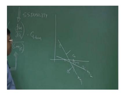
Then, the requirement for delta e also will reduce, which we have seen just few minute back, we did that suppose there is a aircraft X C g 1 and this the aircraft X C g 2, which is statically more stable, definitely I call it one and call it two, which is having more negative slope at the trim at this point.
