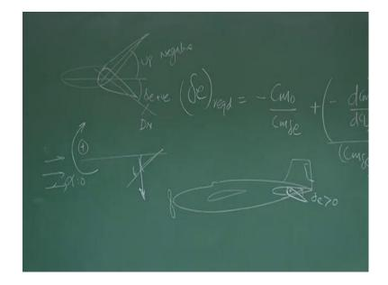
You know primary contributor were tail, if I said the tail at a negative angle setting angle, it will give a positive C M naught that is, if I put the tail like this some setting angle I call I T. So, as flow is coming like this at alpha equal to 0, this will have force generated downward direction and suppose C g, somewhere here of the aircraft. So, this will give a positive pitching moment, which is C M naught. What was the C M delta e? Try to physically understand this.
