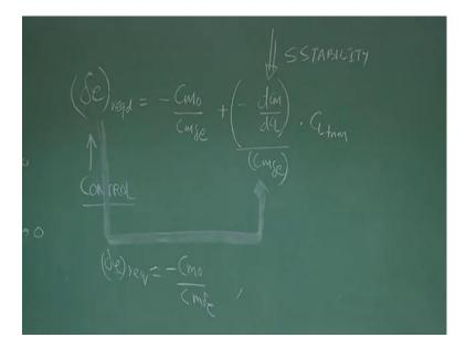
Now, try to visualise the connection between control and static stability, so if I ask you, which part is over control part here, but here naturally control is the elevator. So, this is our control part is a elevator control part to be more precise, which is the stability part here, stability means, what I am talking about static stability and you know d C M by d C L is static stability parameter, so this is the static stability parameter.
