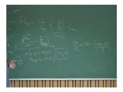
Suppose this is airplane and this is the horizontal tail and this is the elevator, let us say there are wing, whatever it is. What is delta e? Delta e is the elevator deflection and how do you define delta e, sign convention wise this is the delta e positive and delta e up, this
