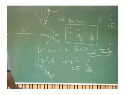
Now, if I substitute this here, so what I get, C D equal to C L into C L by pi aspect ratio e and that is equal to C L square by pi aspect ratio e. So, this is nothing but, C D i, C D induced. So, now, for a wing what we see. For a wing if I want to find total C D, I know total C D will be what. One part is induced because of lift, which is given by C L square by pi aspect ratio e and what about the other part. Suppose, this is the wing or further we might have, this is the airplane.
