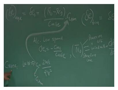
So in a simpler form I can write Delta E trim or required, whatever you use is equal to Delta E0 + N0 bar - XCG bar divided by CM Delta E. And you all know when you say bar means it is non-dimensionalized with mean aerodynamic chord, this is not complete I have to write here CL trim, so what is the message from this relationship we got? If I want to trim an airplane at tail particular CL once I know this, this, this and this I know how much elevator deflection has to be given.
