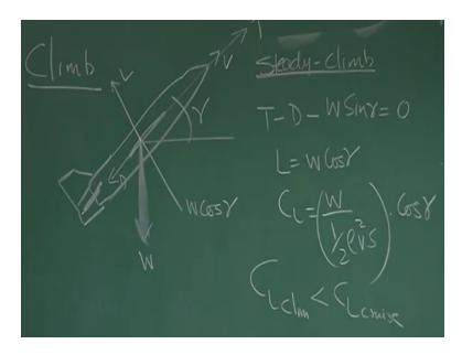
How did you model the climb? if we recall this is the airplane this is vertical tail, this is the horizontal tail, this is the wing and said T this is D and this is Lift, and the V. V in thesame direction, this is W so this is W COS of flight path angle, which is gamma right so how did you
