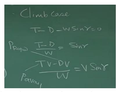
If I take the climb case we have seen T - D - W Sin Gamma equal to 0, so I can write T - D by W equal to sign gamma, or T V - DV by W is equal to V sin gamma. We have already done all these so what is V sin gamma? If this is V, V sin gamma exist component, so this is rate of climb okay this is rate of climb.
