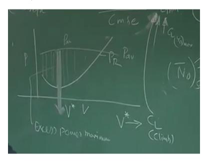
Now from pilot point of view, if you see if I write power and V you know that power required graph will follow something like this, and let's say power available for particular type of engine, propeller driven, let say remain all must constant with speed where ever this excess power is maximum, this is the excess power maximum you really know this is power required is power available.
