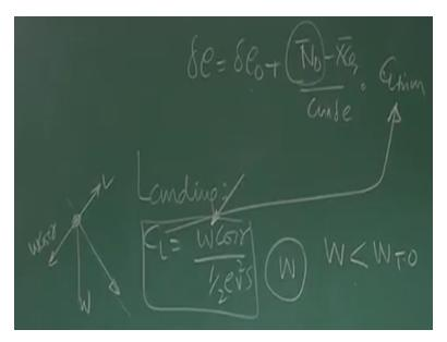
Based on Delta E equal to Delta E0 + N0 bar - XCG bar, by CM Delta E into CL trim, see the landing. During landing, what is happening again the velocity vector is like this, and you want to follow this path. This is the weight, this is the lift, this is the W Cos Gamma, CL will be again W Cos gamma by half row V square S, this is fine.
