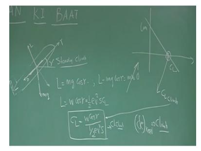
This is the wing, this is the CG, this is your MG acting here or the weight, and here it is drag, here it is thrust, here it is lift. We have assumed that, the thrust axis is along the fuselage reference line, we are also neglecting the angle of attack, or not neglecting we are saying the angle of attack is small, okay. And we are trying to develop a model for steady climb with no acceleration right.
