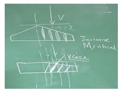
Suppose this is the platform of a wing and these are the way the aerofoil shape has been contoured. And if there is relative air speed V then do I call that this airplane is having a sweep or not? Should I tell this is having a sweep in a literal it says question is yes or no? Let us see what is the physics is behind or philosophy behind the sweep. The understanding was suppose, this is the rectangular wing and this is the free stream relative air speed okay. We understand one thing,
