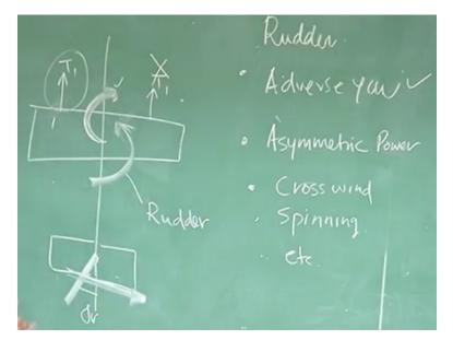
But you understand rudder is required here spinning, sometime the airplane during spinning may go to stall, stall is as the angle of attack may increase very high, your aileron etc., may not be that effective because the wing has stall but rudder can be very effective and that rudder can be used to stop this rolling motion or it can help us in taking out the aircraft from stall. So these are the things that we will be discussing, but you should know that rudder has specific purpose.
