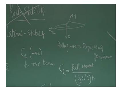
X axis that is, this is the airplane a moving like this a rolling movement is positive is right wing going down clear. Moving like this right wing going down is the rolling movement positive, so rolling movement positive is right wing going down, while I am moving with the airplane right and say for all that examples which we are being discussing, we are discussing in terms, Non-dimensional coefficient.
