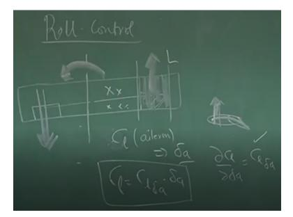
To conclude this part we will now finish our lecture by talking about roll control. We know what was pitch control, pitch control was using elevator. What was yaw control? Yaw control was through rudder, Now we are talking about roll control, that is if you want to bend the airplane right or left, which control surface I will be primarily using, Please understand rolling moment convention is right wing going back is positive, left wing going down is negative right?
