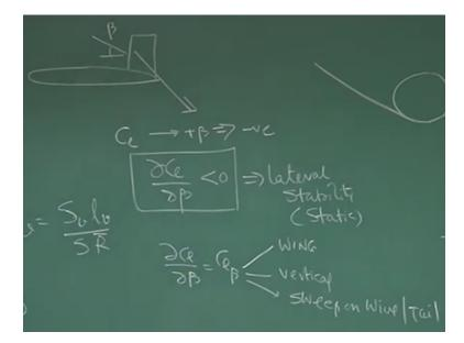
This is the airplane this is the vertical tail and let's say it has banged, it has banged means it is side slipping okay. What type of movement I want if it has banged because of the disturbance I want the movement should be generated which is negative CL should be negative who will generate this movement, this is for the vertical tail because as it banks, it will see starts side slipping so there will be a force active on the vertical tail that is if this is the airplane.
