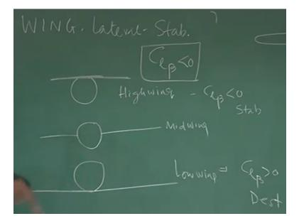
What is the wing contribution for lateral stability? You might be seeing a wing which are having led on the top of the fuselage, these are called high wing. We will have wing set at the middle they are called mid wing configuration and there are wing could be like this these are called low wing. Which one do you think will generate CL beta less than 0? What is our aim?
