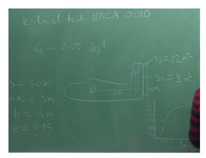
Coming to the next problem, an aircraft has vertical tail having a symmetric aerofoil NACA 0010 with lift come slope of aerofoil 0.09 per degree and the vertical stabilizer area 12 meter square and the rudder area is 3 meter square. And the span of the vertical tail is 4 meter and this aerodynamic center of the vertical tail from the CG of the aircraft is 6 meter and we are given the wing area is 50 meter square.
