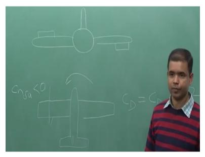
There will be a positive roll, so we can say the CL DELTA A is greater than 0, and next control derivative CN DELTA A for the positive deflection of aileron means right aileron up and left aileron down if I see the front view, this is the front view right aileron up and left aileron down in this case, this wing will feel the more lift, and as you know the CD = CD0 + KCL square and here you can see the CD.
