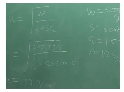
And I can write U is = route over W by half ROW S CL during the landing and if I substitute these values, 5 thousand into 9.8 let as to constant half ROW is given to us 1.2 kg per meter cube, the area is fifty meter square and the CL is 1.5 and from here I will get the value of U, is = 33 meter per second. So now I have this U 3 meter per second and BETA 22 degree from this U and this BETA I can find this velocity the resultant velocity.
