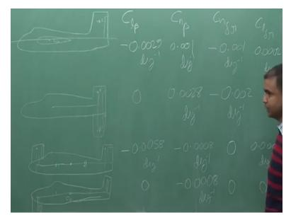
Let us find this is our design suppose, suppose this is the CG the aerodynamic center of the vertical tail is somewhere here this is the body X axis now this is the rudder what will be the value of CL BETA for this design? We can see the contribution of the CL BETA of the vertical tail is -0.0029 per degree and the wing and fuselage contribution to CL BETA is 0.
