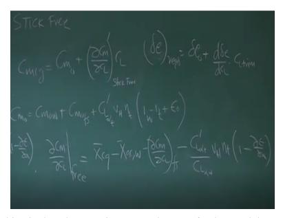
Because of something is slotted XAC wing - DCM by DCL fuselage and then - now CL Alpha T prime will come here CL Alpha wing VH Neeta T one - D epsilon by D Alpha so nothing new we are doing we have agreed. That because you are allowing the floating tendency the stick is not fixed so the elevator will go to a particular Delta E and will set, Delta e float and set will the curvature will change it will be going up like this so CL Alpha tail will change.
