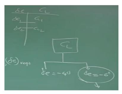
For a given CL this is the Delta E required this CL one Delta E 2 for CL 2 so he will be seeing that how much Delta E required for the particular CL or particular speed from that he develops the field for example for same CL if CL remaining same if one aircraft required Delta E = -4 degree and another aircraft or same CL for same condition which required Delta E = -6 degrees and the pilot understands that the aircraft number 2 is statically more stable.
