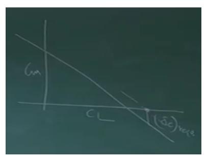
This is governed by simply by this that if I trim it here then I need some Delta E required and that angle if it is 5 degree it has to 5 degree only it as nothing to do is stick fixed or stick free this stick fixed means I take that angle to 5 degree and lock it.
