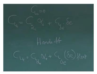
Let us also go back we have till this CLT will be what? CL Alpha tail into Alpha tail + CL Delta E into Delta E, we are assuming that CL 0 is 0 assuming things to be symmetric or polysymmetric. Now, we are assuming CL 0, first let me write this is equal to 0. Now see at trim when hands off or I don't write at trim level, let's say in a hands off condition, what will be the CL?
