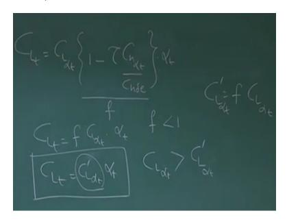
So I can write CL tail as CL Alpha T into one - Tow, CH Alpha T by CH Delta E into Alpha T, when I denote this as F so, I can write CLT = F into CL Alpha tail into Alpha T or further I can write, with the float it is CL Alpha T prime into Alpha T, Note down this, If it was not floating, It was not floating then, it is CLT CL Alpha T into Alpha T because of the floating I have put prime, so that make distinction okay and what is F?
