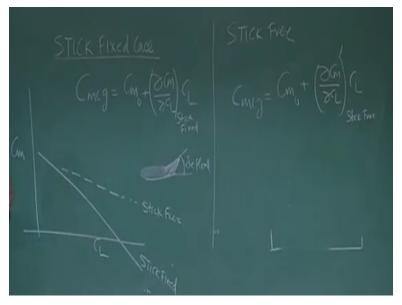
So let us do that, let's see for this stick fixed case, CM CG was CM 0 + DCM by DCL into CL, stick fixed for stick free what will happen? For stick free it will be CM CG will be = CM 0 prime, + DCM by DCL prime into CL. I will for time being I will not bother you with CM 0, focus on DCM by DCL prime, what is the meaning here? It is stick fixed and it is stick free okay,
