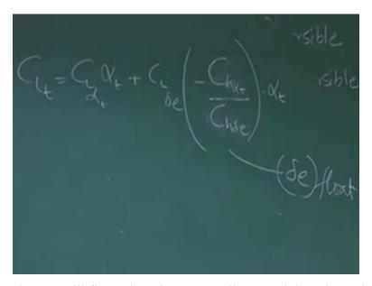
Now how much Delta you will float? that I know CL tail = CL Alpha T into Alpha T + CL Delta E, into for Delta E float I write CH Alpha T by CH Delta E into Alpha T, let me repeat let me repeat again, at Alpha T Delta E also will float so, whatever lift or lift coefficient the tail is seeing will be CL Alpha T into Alpha T, + CL Delta E into Delta E float okay.
