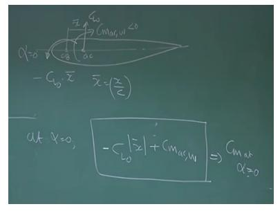
And put this minus sign then no confusion this is the physical distance between AC and CG non dimensionalised with the cord. So that one moment will come at Alpha = zero in addition do not forget because of cambered aerofoil CMAC wing already there so that also will get added so total of this see it will generate a large negative value okay to see that this part is negative this is X is behind CG it is statically stable.
