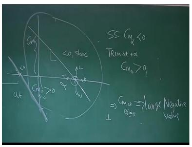
What we look for this can I configure whole airplane so that CM and Alpha variation look like this that is its slope is negative so statically stable slope is negative slope so statically stable and CM at Alpha = 0 which you called CM0 is greater than zero what is the advantage here this
