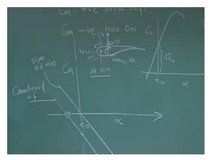
So I if I want fly cruise I want the moment should be zero so my trim point for this aerofoil configuration is this for symmetric it is this for symmetric unfortunately Alpha = 0 so I will not (()) (26:13) be able produce any lift so this is meaningless for me for cambered theoretically speaking some lift to generate because of some angle here but that is not a good way of flying when you have velocities so this is also not accepted for us.
