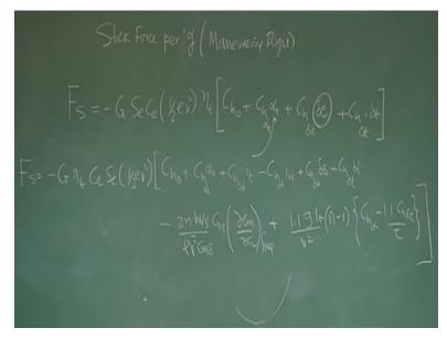
Once you put that what happens once you put you will get the expression like this FS = -GNeeta T CE SE half ROW V square CH 0 + CH Alpha T into Alpha 0 + Ch Delta T into IT - CH Alpha into IW + Ch Delta E into Delta E 0 + CH Delta T into Delta T - 2 N W by S ROW V square Cm Delta into CH Delta DCM by DCL free + 1 point 1 G LT by V square Into N - 1 in bracket it is CH Alpha - 1 point 1, - CH Delta E by Tow this will be the expression. This is very mechanical
