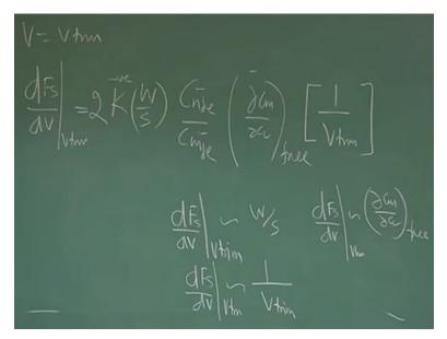
So, at V = V trim we will get DFS by DV at V trim will be = K W by S, CH Delta E by CM Delta E DCM by DCL free into 1 by V trim or I put 2 here, this is the expression so, what is the physical interpretation of this. If I want to find out this gradient, then I know that for a lightly loaded airplane that is whose wing loading is less like gliders and all, DFS by DV also will go down okay. Also you know that.
