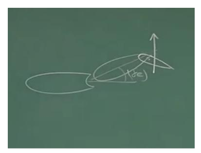
The mechanism we have already discussed suppose the elevator has to be kept at this angle for trimming at the particular CL, and you want doing it by pulling the stick, you are trimming at
