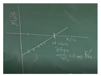
So now I will plot DFS by Q by DCL and XCG location here, So for 1 CG location I am getting value here second here, third here, 4th here, fifth here join them what is this point, This point is the XCG location at which DFS by Q by DCL is 0. So this is the CG location which we are talking about stick free neutral point, clear. DFS by DQ by DCL which is the slope of each of this line, I am cross plotting them with CG.
