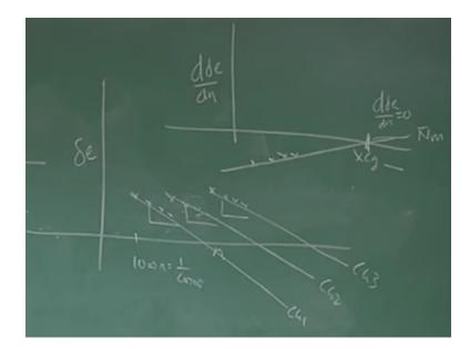
So what I have to do very simple, I will again Delta E and N I will see that for different N, whatever I am measuring ,That I am computing using 1 by COS PI right. I generate this straight line, this is CG 1 and another set for CG 2, and another set CG 3 up to CG 5 that is what I am doing, I am for the CG 1 combination 1 flight, What is the Delta E I am measured, I put it here and what is the load factor I am getting because of different bank angle, for 10 degree some Delta E.
