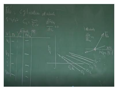
So I can write to find N0 prime, I can write it is the CG location, this is for experimental purpose at which DFS by Q by DCL is, how do I do the experiment? When I am going for when Pin point experiment, I go to in altitude again note down altitude, I note down also at the temperature because this are required measuring the density. I trim my airplane for V 1, V 2 up to V 5 I get I measure FS, for every trim I measure the what is the stick force.
