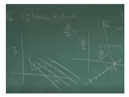
Say NM prime is that CG location at which DFS by DN = 0, there is no problem in that. We have already, measured FS through our stick using the strain gages, so I will plot again FS VS N for different different CG location, as you have d1 for Delta E, then I take the slope, I plot DFS by DN VS XCG and 5 6 point I will get, join them and this is the CG location, and the CG location at which DFS by DN = 0, so this is NM Prime.
