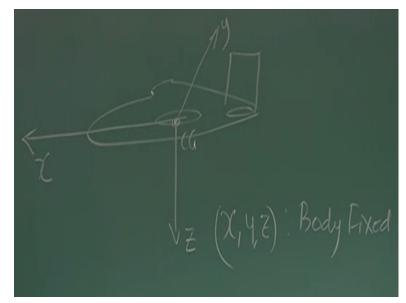
If I draw an airplane I preset the axis system and I am talking about an axis system is X Y Z which is body fixed X Y Z so, body fixed and located at center of gravity this point is at center of gravity. Now it depends on the purpose how do I align this axis there are many ways you can align this axis for many, many exclusive purposes but here to start in the simplistic manner, we are allying this X axis let say on the fuselage reference line this line on symmetric may not be guaranteed.
