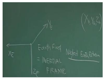
Now let me defined another axis system which is earth fixed this closely I can say this is inertial frame I will explain you what it let me write this then I will come back to this so, completion of this drawing let me write this is an earth fixed and inertial frame of reference I will talked about it do not worry. What is happening you see when I try to write the equation of motion if I through a body.
