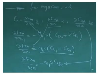
We have written as d fx a by du b y u1 into u by u1 plus d fx a by d alpha into alpha plus d fx a by d delta e into delta e of course this term is aerodynamic force that I have been telling you repeatedly similar expression you can do for thrust expression also. At once you know how to do for aerodynamic and you know how to encounter thrust effect also.
