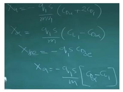
Very simple see from here xu into u that means this whole team is xu that is xu is minus q1 s by m u 1 into cdu plus 2 cd1 right. And you know u 1 is the steady state velocity at cruise because all the equilibrium in steady state is at cruise. So nearly you are smart enough to tell me what is x alpha? X alpha you can check yourself. X alpha will be q1 s by m c l minus cd alpha as simple as that okay. So X delta will be what? X delta will be minus q1 s cd delta e ok.
