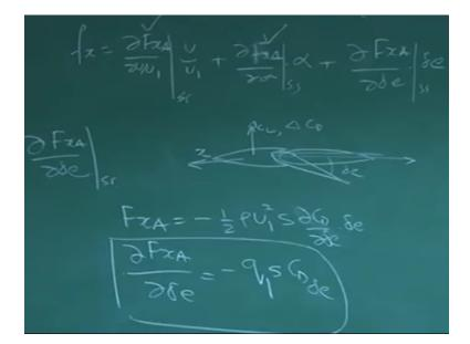
So let us again come back that what we have fx equal to f d fx a by du by u1 u by u1 plus d f d fx a by d alpha into alpha plus d fx a by d delta e into delta e we have already evaluated this evaluated this we know this have to be evaluated at steady state we have known left with evaluated at steady state.
