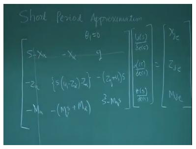
This is our standard equation s minus x u minus x alpha g and the minus zu then s and then u1g minus z alpha dot minus z alpha then minus z q + u1 into s and minus m u minus m alpha dot s + m alpha then s square minuses mqs this of course into u of s alpha of s theta of s equal to x delta e and z delta e m delta e you write it like this theta e by delta e. We should note down that we are note writing q here.
