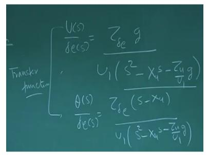
If I do this then I find from this u of s /delta e(s)=z delta e g / u1g of s square -x u s - zu / u1gand the theta of s/ delta e of s = z delta e int s - x u / u1g int s square -x u s - zu / u what is u of delta x and delta a is a transfer function from the short period of you know that is alpha e and delta e delta was a transfer function it was a transfer function okay.
