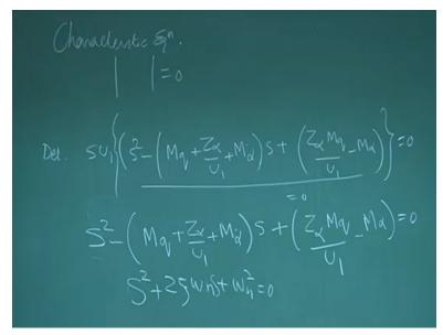
Now we are looking for the characteristic equations and that will be determinant of this = 0 and that will be give me the result something. Like this determinant is su1 s square minus m q + z alpha by u1g + m alpha dot s + z alpha m q / u1g minus m alpha that will be equal to this is on this one is here and here and this equal to 0 right. This equal to 0 means this one is 0 or this one is 0 or this unit some this whole term = 0.
