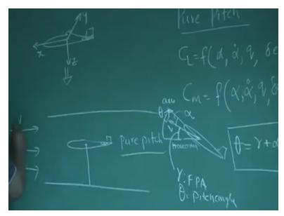
Pure pitch is about y axis and this positive pitch nose is going up and negative pitch going down like this, so it has pitch rate q positive q negative ok. And we know by now that c l is function of alpha, alpha dot, q, delta e right.
