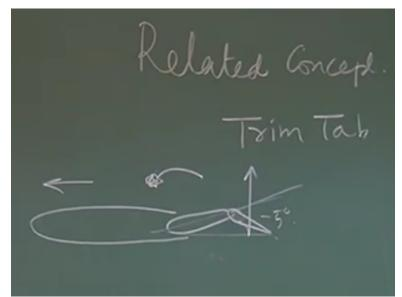
So related concept to stick free is trim tab if you now realize that this is the tail so this is the elevator and put it trim tab like this, what happens suppose you do not put the trim tab here if I have to fly at minus 5 degree elevator. Please understand where the elevator minus 5 degree is required. So what the pilot will do.
