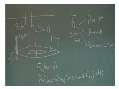
N not stick fixed whether I should take power on and take power off or propeller wind milling this questions where there right. Physically understand you know this is the airplane suppose you estimate neutral point stick fixed and let say this end point is some where here this is the end point when you compute n not bar let us say that we have not taken the contribution of engine ok right. That is this and we will say that power off typically glide without an engine.
