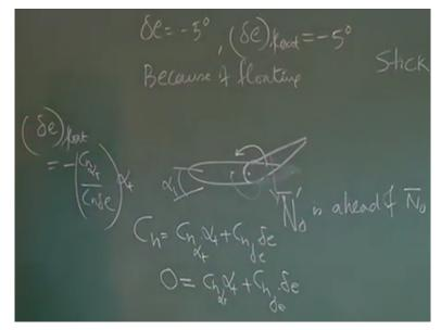
We are assuming that at the given alpha t the elevator has already floated like this and that why c l alpha of the tail reduces and that why neutral point is stick free is ahead of neutral point stick fixed because it float at the particular equilibrium so the c l alpha tail is reduced ok. That is why neutral point stick free is ahead of neutral point stick fixed and this condition is taken as first equilibrium point from here we take to the next one.
