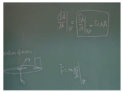
So you had a motivation for work in body frame this two reasons and how to do that need to work in inertial frame but we have motivation to work in body fixed frame so what is the trick you said after all d v by d t is the vector differentiation so we use this relationship d a by d t in inertial frame is equal to d a by d t in body frame plus omega cross A right.
