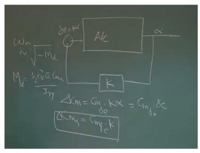
Similar thing you have to do for natural frequency you have to change natural frequency what we have to do? This is the aircraft this is alpha you tab alpha this is k and again delta is there for k alpha that goes to the plot so what happens I write delta c m equal to c m delta e into k alpha because it is nothing but c m delta e into delta e and delta e is k alpha.
