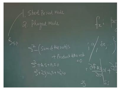
What is the short period mode, short period mode will correspond to this because this real term is large negative and typically if the airplane is moving like a cruse if I give a short elevator input one mode will be like this it will really come back to equilibrium it is the transient so that is the short period mode. Phugoid mode is if I exit phugoid mode is when I hold the elevator for long the airplane will come back to equilibrium.
