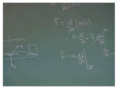
Lot of question was if I am trying to write the equations of motion in inertial frame that means what will happen. So we know that F is d by d t rate of change of momentum. And we know nothing but m d v by d t plus v d m by d t so another approximate value. As said we will neglect the second term and as if we assumed as d m by d t is zero but you know the air craft has fuel and there is huge fuel consumption.
