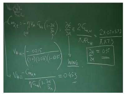
And we have the formula, CM Alpha tail which already we know Neeta VH CL Alpha tail into 1 - D Epsilon by D Alpha okay. Let me repeat again this is CM Alpha tail which is Neeta for this example we will take Neeta as 1 VH is tail volume ratio CL alpha tail is the lift cut slope of the tail based on the tail area and D Esilon by D Alpha is the downwash gradient and you know already in first course you have seen D Epsilon by D Alpha I can compute as CL Alpha wing by  $\pi$  aspect ratio.
