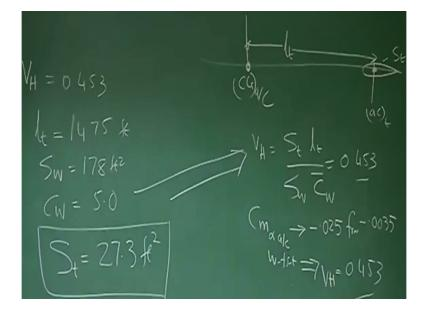
Remember if this is the central line of the airplane, and if this is the CG of the aircraft and if this is the tail, and this is the AC of the tail, right and this is the S tail area, then this distance is called tail moment on the horizontal tail LT and if you see LT here is 14.75 feet okay. And then what is VH? How VH is define? VH is defined as ST into LT by wing area into mean aerodynamic chord of the wing. So this ratio ST LT by ASW for this problem is 0.453.
