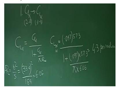
So the contribution of wing towards stability or to CM Alpha will be stabilizing or destabilizing we know that for it to give stabilizing effect, the AC should be behind CG right.
