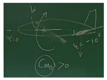
If you again recall one of my lecture I have explained this. If this is the fuselage reference line, the wing is set at some angle with fuslage reference line. This is called IW or wing setting angle okay and that wing setting angle is  $1^{0}$ .
