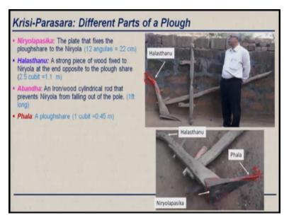
And Niryolapasika that is the plate fixed the ploughshare, this is the portion Niryolapasika, right and of course this whatever I am showing is made of Iron right. But earlier days and even today also in some parts of the country this is made of wood right this Niryolapasika and which is around twenty two centimeters in length and of course if you go to some other book there also what is the width and everything is given not in this case Krisi-Parasara.
