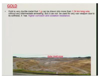
So, if you look at Gold, Gold is a very very ductile metal and it has a higher corrosion and oxidation resistance. One gram of Gold can be drawn into more than 1.24 km long wire without any intermediate annealing. So, that is why it has been used very easily for jewelleries, very nice jewellery you can find even today although it was being done earlier
