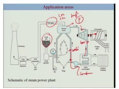
This is at high pressure and what are the remaining gases such as CO2, S2 and SO4 goes as part of the flue gas or also the high pressure you pass through a turbine, turbine with extends and thus some work the work gets converted into electricity through generator and the remaining low pressure steam gets condensed and then recycled here.
