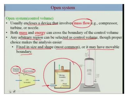
So, but they are other examples where you need to consider flow. Where mass need to also transfer from the system to the surrounding and this is the common occurrence in a engineering applications such as turbine, compressor or nozzles and this is, so this kind of devices involves mass flow and in such case both mass and energy can cross the boundary of the control volume okay.
