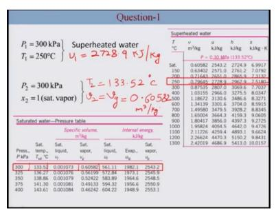
So, we need to look into superheated water table. In superheated water table at 250 degree Celsius and 300kilopascal which is equivalent to 0.3 mega Pascal. The values are these to the value of internal energy U 1 is 2728.9kilojoule per kg. In state 2, it is mentioned in the question that water is a saturated vapor and the pressure is same as initial pressure.
