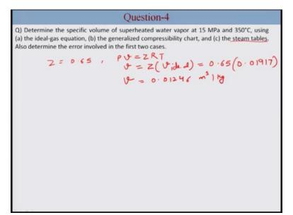
So now we have Z is equal to 0.65. We can apply the equation that is P v is equal to Z R T. This is also v is equal to Z multiplied by v, from the ideal gas equation which we have obtained earlier. So, this value is 0.65 multiplied by 0.01917, so the value of v is 0.01246 meter cube per kg. We also have to calculate the error involved in the two compare to this steam values to the steam table.
