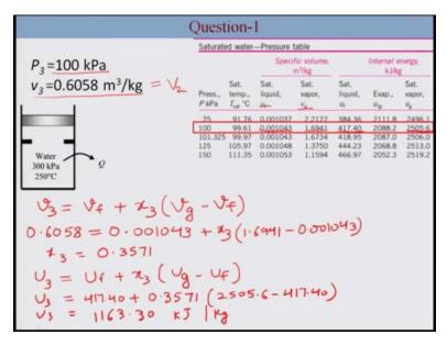
Next it is said that, now the piston rest on this stops and so it means that the volume of the piston cylinder device it is not changing and pressure is now decreasing. So, pressure reduces to 100kilopascal and the volume or specific volume is constant because mass is not changing overall volume is not changing.
