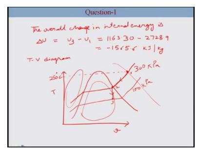
So, the overall change in internal energy is delta U which is equal to U 3 minus U 1, U 3 is as we have calculated 1163.30 and U 1 is 2728.9. So, this is equal to minus 1565.6 kilojoule per kg. Internal energy of the system is decreasing. Now we also had to plot T v diagram, so if we think what we have done this is T and v these are the saturation lines.
