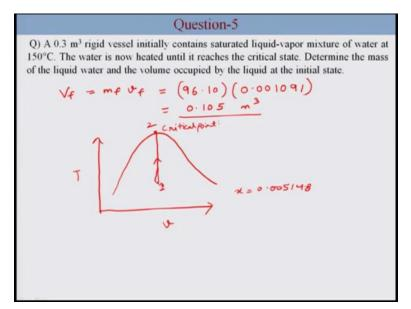
To calculate the volume occupied by the liquid v f is equal to mass of the liquid do specific volume of the liquid. So, mass of liquid is 96.10 and the specific volume of the liquid is 0.001091. So this is equal to 0.105 meter cube, so this is the initial volume occupied by the liquid.
