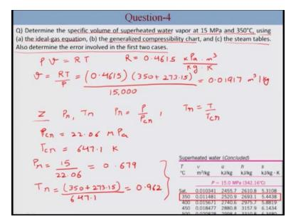
Moving to the next question in question 4, determine this specific volume of superheated water vapor at 15megapascal and 350 degree Celsius using the ideal gas equation is generalized compressibility chart and this steam tables also determine the error involved in the first two cases.
