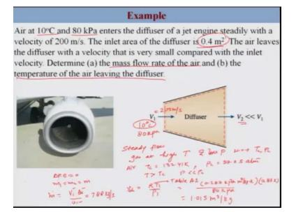
So this is your 20 kelvin or 20 degree Celsius, okay and so there is a increase in the temperature at the outlet condition and the reason being is that your kinetic energy of the air gets converted to the internal energy and raising the temperature of the overall air. So let us now take a look at different device, okay so we have discussed diffuser and nozzles now we are going to discuss turbine and compressor.
