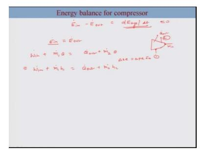
So let us start with this a generalize energy balance here, okay so we will consider this to be 0 because again the compressor will be considered as a steady flow device, let us say you have this inlet fluid and this is outlet and there is a work which is supplied let us say a shaft work, okay and there is some heat loss. So this could be your out, okay so we can write this generalized energy balance for the control volume for the steady flow condition as follows, okay.
