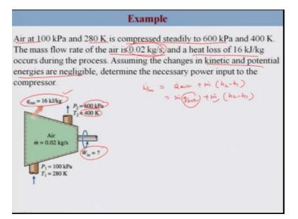
So this is how you are going to solve such a problem for the case of compressor, so what is important here is that if you look at carefully the work here which is being supplied to the compressor or to the control volume has raised the temperature in and essentially it also as increased the enthalpy where enthalpy at the outlet condition is much higher than the inlet condition, okay. So this is your increase in enthalpy due to mechanical energy input, okay.
