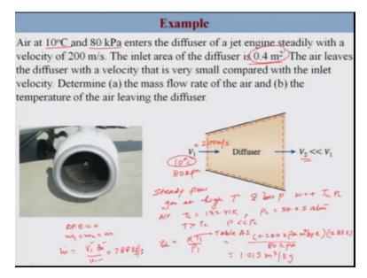
So this is our basic energy balance for nozzle and we can make use this analysis for a specific example, so let us take that example this is a case of a diffuser for jet engine. So what we have is air which is at 10 degree Celsius and 80 kilo Pascal enters a diffuser, okay so this is your 10 degree Celsius and 80 kilo Pascal.
