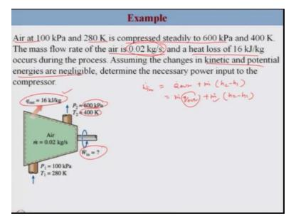
So this is what we are going to write here m dot Qout which is already given here because this is given to you plus m dot h2 minus h1. Now so what we have is we have been given m dot which is of course 0.02 kg per second. Qout is given to you we have to find h2 minus h1.
