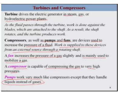
Turbine we have already looked at a bit in early stage of this course basically the purpose of the turbine is it drives the electric generator in steam, gas or hydroelectric power plants. So during in the turbine the fluid pass through the blade of the turbine, okay and it does work against the blade blade is connected to the shaft so it rotates the shaft and thus it produces work. So that is the philosophy or that is the purpose of the turbine in that case.
