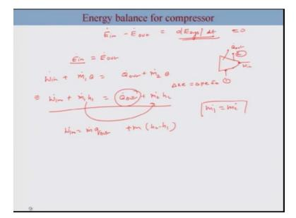
So this can be written by taking it here okay and then you can write it Win as simply m h2 minus h1 considering that m1 dot is equal to m2 dot okay because of the single stream, you can also further simplify this and or use Q in terms in the units of kilo joules per kg by considering m dot multiply by Q dot, okay.
