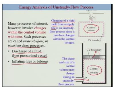
Ok, so now we will look at the systems which are considered as unsteady flow processes because there are many processes of interest which involves changes in the control volume properties. So for example, you have charging of a rigid tank from a supply line unsteady flow condition which essentially means that the control volume properties or the control volume undergoes changes with time and such kind of changes would be a part of unsteady flow process.
