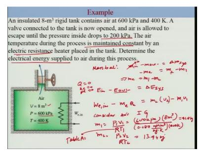
So this is an example of insulated 8 metre cube volume, ok which contains air at 600 kilo Pascal at a temperature of 400 Kelvin and there is a discharge value open the specific valve and there is a discharge in the pressure starts dropping drops to 200 kilo Pascal. The temperature of this particular air is maintained constant by an electrical resistor and what we have to determine is electrical energy supplied to air during this process.
