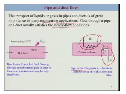
So Pipe and duct flow are very common in our daily usage and is very important in many Engineering applications. So a simple flow through a pipe usually satisfy the steady flow condition. This is an example of a hot flowing through a pipe and the heat transfer in such a condition are quite significant.
