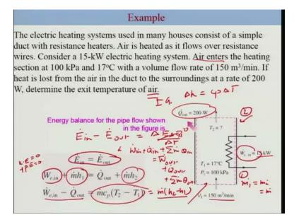
So this is an example of an electrical heating system which is used in many houses, ok? So you have a simple duct with a resistance heater. Ok? and there is a electrical work of power of 15 kW which is supplied to the flowing fluid and this is air which enters here at 150 meter cubed per minute at 17 degree celsius with a certain volume rate which is of course 150 meter cube minute. And there is a heat loss of 200 Watt and what we need to find is the exact temperature of the air.
