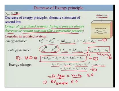
So in another word, what we are saying is Exergy of an isolated system during a process always decrease or remain constant for a reversible process. So we can try to derive this so we consider a isolated system okay for which the energy balance would be simply delta E system is 0 because there is no in there is no out okay because there is no heat, work or mass transfer and thus E2 is equal to E1.
