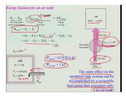
Now we can take another example which is Exergy balance of an air tank. Okay and this problem is following. So you have insulate tank with air and there is a shaft which is applied and the outside temperature is 20 degree Celsius so what has been done is it has been asked to do certain work in order to raise the temperature to 54 degree Celsius so what we can do is or it's been asked to find out what is the corresponding reversible work for this process.
