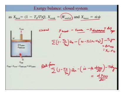
Now, (ex) Exergy of the heat is now very clear that we write in this form. Exergy of work would be useful. Now this would be your W for shaft and electrical work otherwise this will be your W minus W boundary. For the boundary work (I) or where the system involves boundary work and this X mass is simply mass (temp) your Exergy of the flowing fluid okay.
