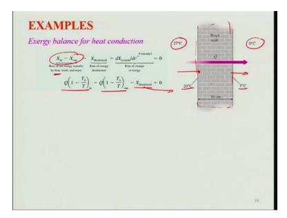
We can do certain examples, now in order to demonstrate this exercise for the Exergy balance so this is Exergy balance for heat conduction, the atmosphere on the left on the brick is 27, this could be your room and this is your outside temperature which is 0 degree. At the wall, it is 20 degree celsius and this is at 5.
