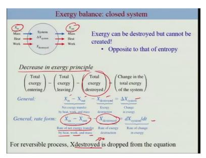
So this is the schematic representation of the system. So we have Xin Xout due to mass, heat,
