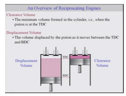
Okay and this volume which is left is called nothing but the clearance volume okay and the volume which you can displace is from BDC to TDC is nothing but the displacement volume.
