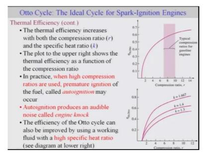
This is a typical range for the gasoline engine somewhere from 7 to 10 and as I said, you can increase the efficiency by increasing the heat capacity which essentially means that you can use working fluid with a higher specific hear ratio in order to have higher efficiency of otto cycle okay. So you can make use of this analysis of ideal otto cycle based on air standard
