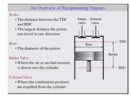
So this means this piston keeps moving from the BDC to TDC and the length of this TDC and BDC would be or the difference between TDC and BDC is basically nothing but the one stroke. So this is the stroke is nothing but the largest distance of the piston which can travel in one direction okay. The diameter is called bore so as I already mentioned, the inlet valve and exhaust valve, now at the, if you take this piston to the TDC, there is certain volume which is also left.
