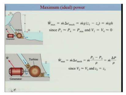
So, we can take an example and apply this aspect, now in cases of an ideal hydraulic turbine, what would be the maximum power. So, assuming that this is the case where you have ideal hydraulic turbine connected with the ideal generator and it means there is no loss of energy had we having here. So, whatever the mechanic energy of the fluid is transferred to the work done by the generator, so this the maximum power okay will be simply m dot e delta e mech.
