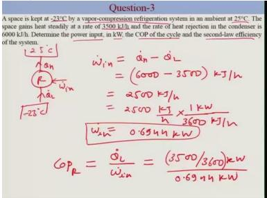
A space is kept at minus 23 degree centigrade by a vapor compression refrigeration system in an ambient at 25 degree centigrade. The space gains heat steadily at the rate of 3500 kilo joule per hour and the rate of the heat rejection is 6000 kilo joule per hour. Determine the power input in kilowatt, the COP of the cycle and the second law efficiency okay.
