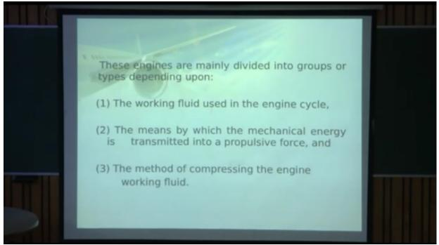
So the engines they were mainly divided into groups or types depending upon the type of fluid used in the engine the means by which the mechanical energy is transmitted into the propulsive force, and the methods of compressing the engine working fluid.
