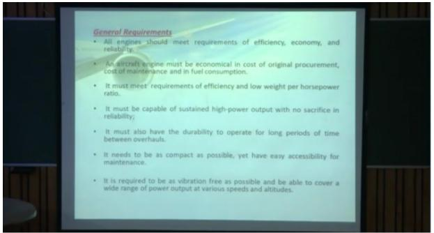
Coming to the general requirements of the engine, what are the general requirements for an engine? The engine should meet requirements of efficiency, economy and reliability, so all engines they should need to be very efficient, very economical, and very reliable.
