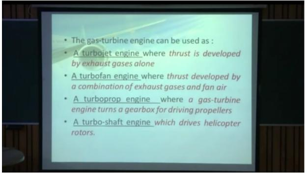
The gas turbine engines can be used as a turbo jet engine, a turbofan engine, a turboprop engine or a turbo shaft engine, so you can see the gas turbine engine, the same gas turbine engines they can be used as turbojet engines, turbofan, turboprop, turbo-shaft.
