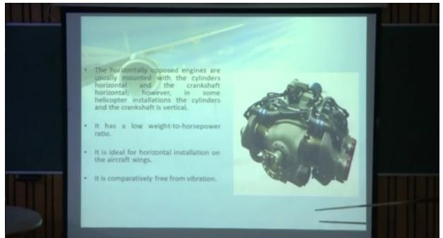
cylinders are opposed to each other so they are called horizontally opposed engines are usually mounted with the cylinders horizontal, the cylinders are horizontal and the crankshaft is also horizontal.
