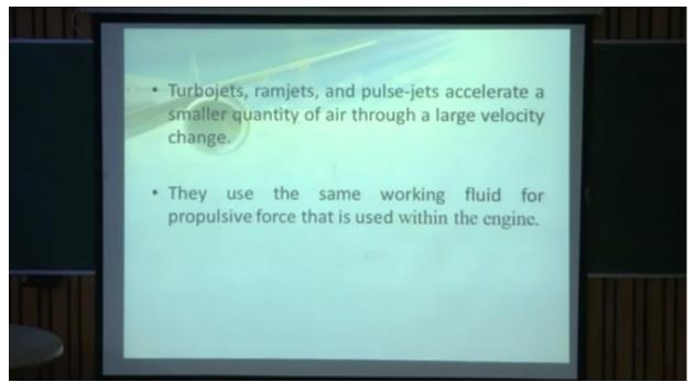
turbojets, ramjets and pulse jets accelerate a smaller quantity of air through a large velocity change, so you have seen in case of reciprocating engines and turboprop engines the air is used in larger quantity with a small velocity change, whereas in turbojets, ramjets and pulsejets they accelerate a small quantity of air through a large velocity change. They use the same working fluid for propulsive force that is used within engine.
