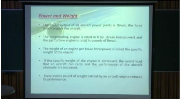
as we have seen earlier the basic requirement of any engine is low weight and high horsepower requirement or high power requirement, so the engines they need to produce force which propels the aircraft forward you need more power and you need less weight, the reciprocating engines, the piston engines, they are rated in B.HP, that is the brake horsepower and the gas turbine engines, the jet engines they are rated in pounds of thrust.
