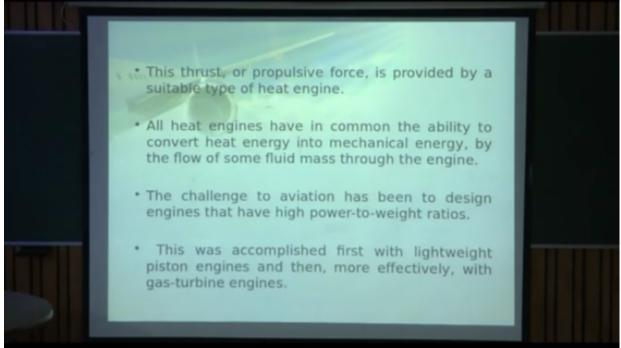
so this thrust which is equal and opposite to the drag is the propulsive force which the force, which moves the aircraft ahead this is provided by a type of heat engine.
