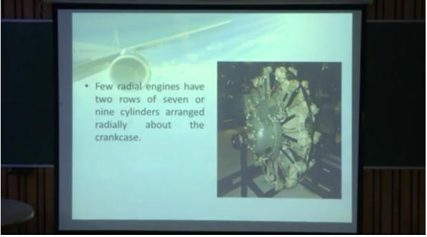
Few radial engines have 2 rows or 7 or 9 cylinders arranged radially about the crank case.
