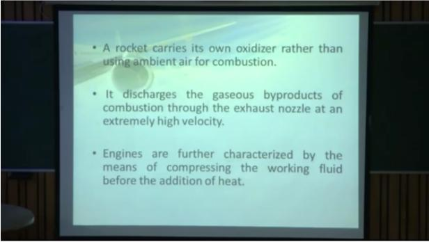
In case of rockets it carries its own oxidizer rather than using ambient air for combustion. The rocket will discharge the gaseous byproducts of combustion through the exhaust nozzle at an
