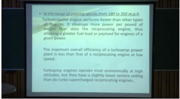
you can use piston engines with superchargers and high altitudes and in the speed of 180 to 350 miles per hour you can use turboprop engines.
