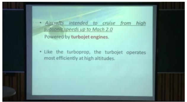
Now for very high speeds where the aircrafts are intended to cruise from high subsonic speeds up to Mach 2.0, you have aircrafts which are powered by turbojet engines. As the turboprop engines, turbojet engines also operate most efficiently at higher altitudes and high speeds, so high speeds and high altitudes you can use turbojet engines low speeds and low altitudes you can use piston engines, low speeds, high altitudes,
