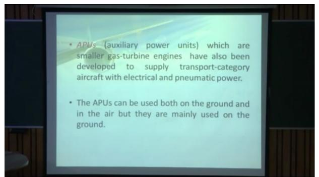
Auxiliary power units we call them APU's, they are small gas turbine engines, they have been developed to supply transport category aircraft, bigger aircrafts with electrical power and pneumatic power, they can be used both on ground and in air but are being mainly used on the ground.
