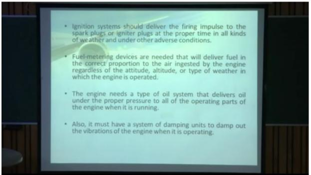
The ignition system should be very reliable, it should be able to deliver the spark, the firing impulse to the spark plugs in all kinds of weather, in all kinds of conditions at the proper time at which the spark is required.
