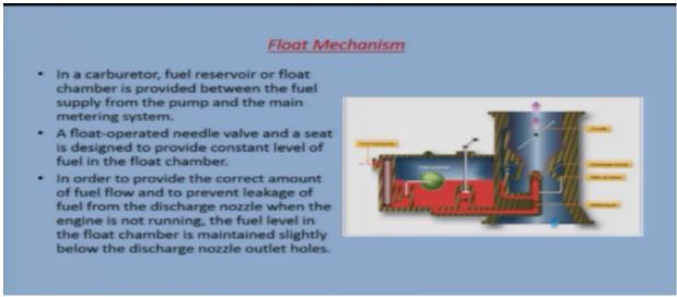
so this is your fuel supply from the pump and this is your main metering system, so this fuel reservoir or the fuel float chamber is between the supply from the pump and the main metering.
