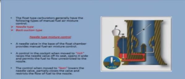
Now the float type carburetors, they are the basic type carburetors they generally have the following types of manual fuel air mixture control, a needle type and a back suction type, so there are mainly two types of mixture controls being used in basic float type carburetors are
