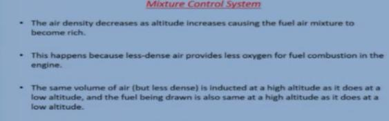
This richness of the mixture at altitudes can be controlled either by a manual or an automatic mixture control.
