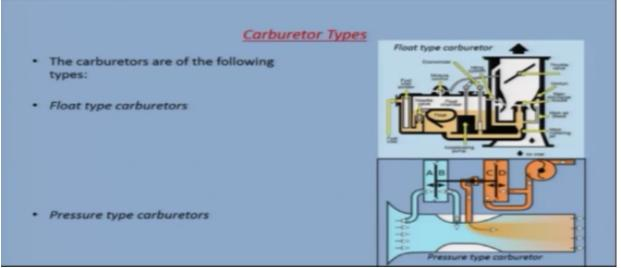
Now let us see what are the different types of carburetors? The carburetors are of the following types, float type carburetors, pressure type carburetors, coming to the float type carburetor. (Refer Slide Time: 05:56)
