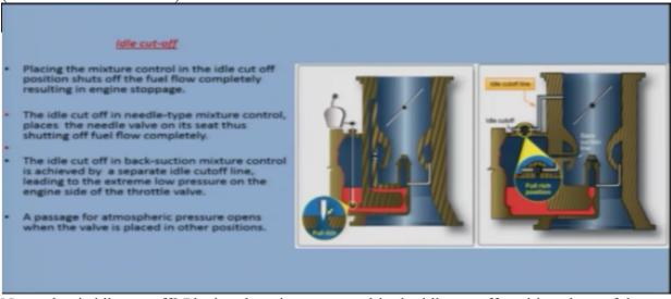
Now what is idle cut-off? Placing the mixture control in the idle cut off position shuts of the fuel flow completely resulting in engine stoppage, so when we have to stop the engine the fuel mixture control, fuel air mixture control is moved to the idle cut off position, in that position the fuel supply is shut off and the engine comes to a stop.
