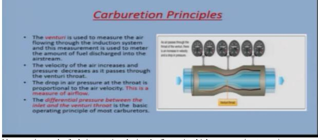
Now coming to the fuel air metering device the first unit which we are going to see is a carburetor, let us see what are the basic carburetion principles being used in a carburetor, you all know about the venturi, the venturi is used to measure the air flowing through the induction system, and this measurement is used to metered the amount of fuel discharge into the airstream.
