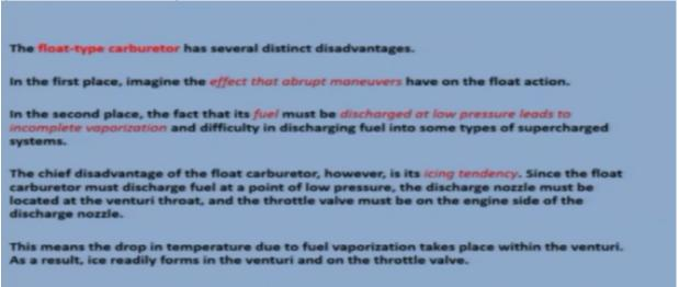
Now we have seen about the float type carburetor, the float type carburetor it is a basically a simple carburetor, but there are various disadvantages also in this carburetor, the first is there are effects on the float, because of the abrupt maneuvers, the floats get affected.
