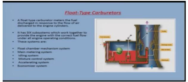
A float type carburetor meters the fuel discharged in response to the flow of air delivered to the engine cylinders, since this carburetor this is a fuel air metering unit, so in response to the air the carburetor has to meter the fuel and deliver it to the cylinders, it has six subsystems which work together to provide the engine with the correct fuel flow under all engine operating conditions.
