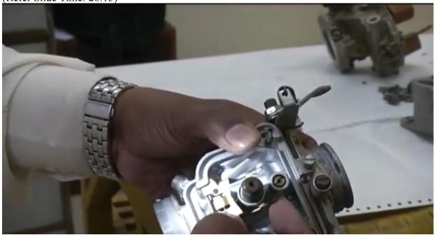
this is the arm this moves like this, there is a needle seat, I'll remove this, see this is removed and this arm is removed, and you can see here this is your float arm and this is your needle seat
