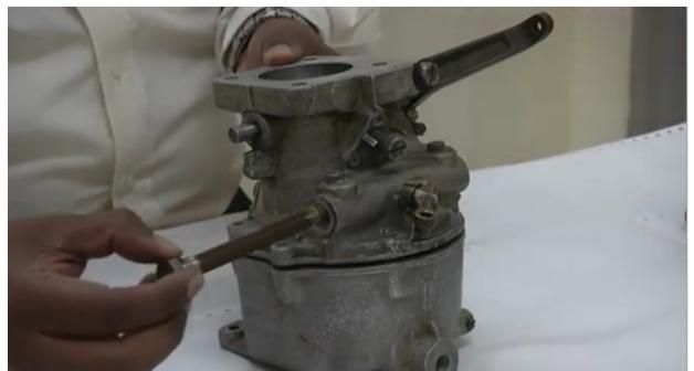
you can see here this is your strainer which will filter the fuel coming inside the carburetor, so inlet, fuel inlet and a strainer, inlet fuel coming from the engine driven fuel pump getting filtered here.
