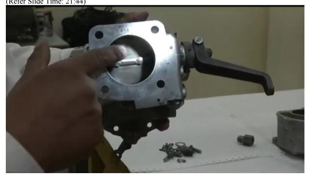
now when the throttle is in the almost closed condition the velocity of air or rather we can say the pressure differential or the fuel metering force is not sufficient to bring fuel for combustion in the idle condition, in that case the fuel is supplied through these holes you can see there is a hole here, you can see small holes on one side of the valve, (Refer Slide Time: 22:17)
