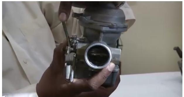
now here you can see the movement of the disk, this condition this is your full throttle condition where your disk is completely open, you can see here the disk, the throttle disk is completely open.
