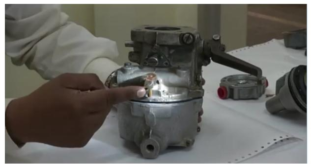
this lever this is your mixture control, this is your rich side R is here, and this is your lean side you can see L written here, so this is your mixture control, this control is also moved with the control in the cockpit, so when you move the mixture control from the cockpit this is mechanically connected to that control and this will move and they will move to the rich or the lean condition as per the selection of the control.
