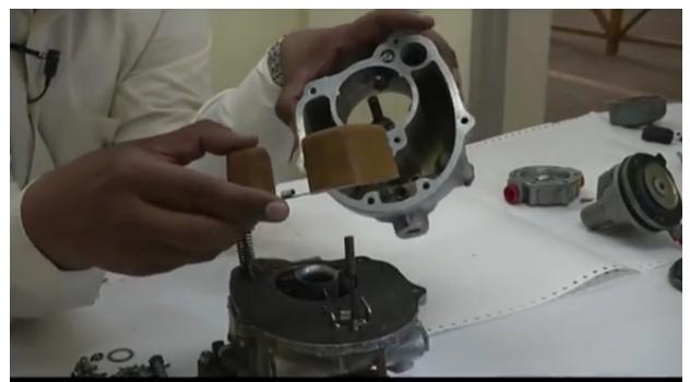
now when the float chamber is empty when there is no fuel in the float chamber these floats they move down, when they move down this will pull the needle valve up, when the needle valve moves up the passage, the fuel passage for the float chamber it opens and the fuel fills in this float chamber.
