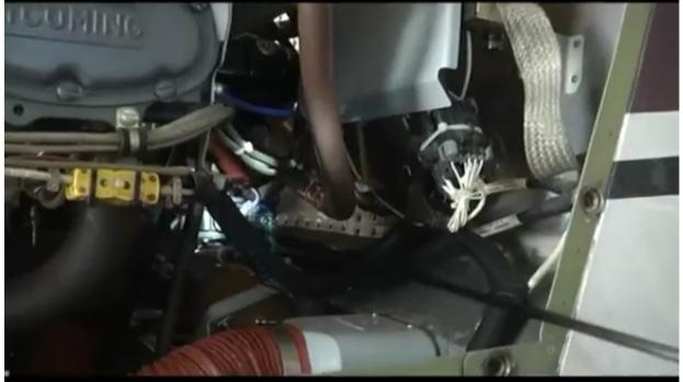
you see this is your engine driven fuel pump, the engine driven fuel pump you can see here, this is your engine driven fuel pump, this engine driven fuel pump will now pump the fuel, the fuel metering unit, this engine which is Lycoming IO-540 engine, the fuel from the engine driven fuel pump is coming to the fuel air metering unit, (Refer Slide Time: 03:20)
