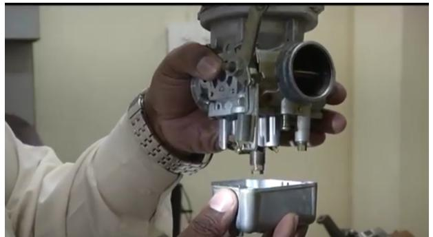
you can see the float chamber here, see the float chamber of this carburetor and these are the floats, you can see the floats.
