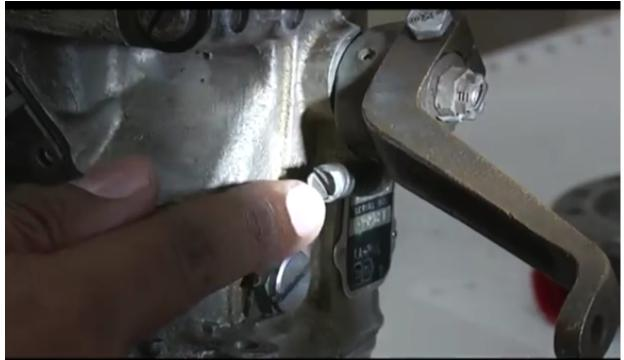
so this is your idle speed adjustment, screw and for idle speed also you need to have your proper mixture, proper mixture of fuel and air so that idle mixture adjustment is done from this condition, this is the needle type valve we have removed it, you can see the valve here, (Refer Slide Time: 13:20)
