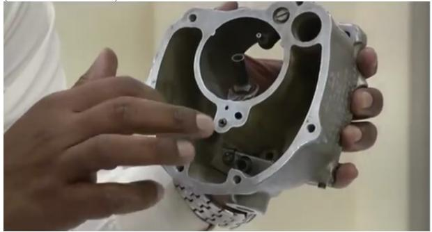
now this main discharge nozzle this protrudes between the venturi throat, this is your venturi throat where the low pressure is acting, so now when the air is flowing through this passage, when the air is flowing through this passage, when this throttle is moving due to the movement of the throttle your air is flowing when you move this throttle this allows air to flow, when this air flows it flows through this opening.
