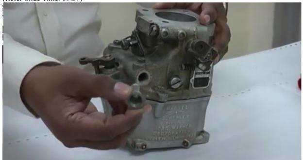
this is the inlet from where the fuel supply comes in from the engine driven fuel pump, the fuel supply comes in through this inlet, this is the inlet point of the fuel in the carburetor, so fuel coming in through this point, now this inlet also has a strainer, (Refer Slide Time: 09:55)
