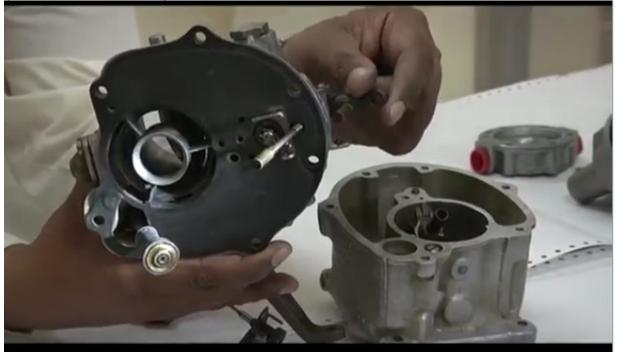
when the mixture control is moved you can see this valve, the movement in this valve.
