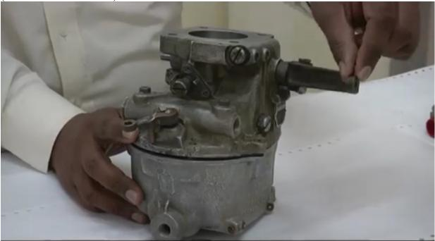
this is your throttle this is connected to the throttle control in the cockpit, so when the control in the cockpit, when the throttle control in the cockpit does moved this linkage via the mechanical linkage this moves, when this moves you can see here in the front there is a butterfly valve here
