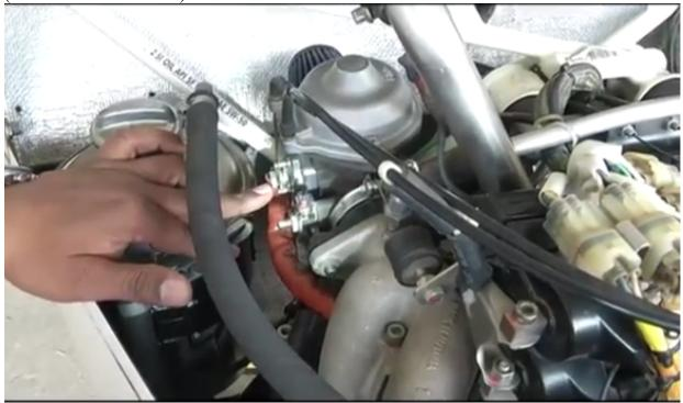
the choke is being operated and this is another extreme, so you've seen an injector, you have seen a carburetor installed on the engine, we will now see how a dismantled carburetor looks like, we will see different types of carburetors and how do they look like, what are the different parts of the carburetors.
