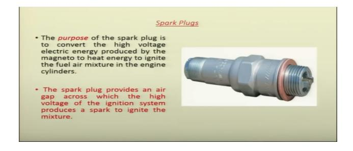
Coming to spark plugs. The purpose of the spark plug is to convert, the high voltage electric energy produced by the magneto, to heat energy, to ignite the fuel air mixture in the engine cylinders. So, the high voltage energy, electric energy, which is produced by the magnetos, this will be converted to heat
