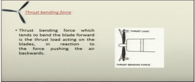
Next is your thrust bending force. First bending force which tends to bend the blade forward is the thrust load, acting on the blades. We all know that, the thrust is acting in the forward direction and because of these thrust loads, the blade, it will tend to Bank the blade forward, in reaction to the forces pushing the air backwards. So thrust bending force, they are they tend to bend the blades, forward in reaction to the force, pushing the air backwards.
