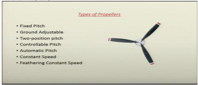
Now, coming to the types of propellers, there are various types of propellers, some of them are fixed pitch propellers, ground adjustable propellers, two position pitch propellers, controllable pitch propellers, automatic pitch, constant speed, feathering constant speed. So, number of types of propellers, let us see them, one by one.
