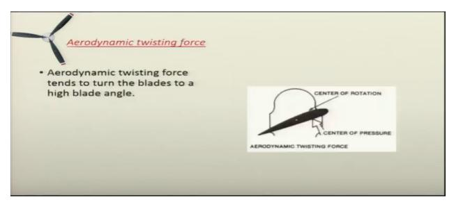
Next is aerodynamic twisting force. We tend to turn the blades to a high blade angle. So, this aerodynamic twisting force will tend to turn the blade, to a higher blade angle.
