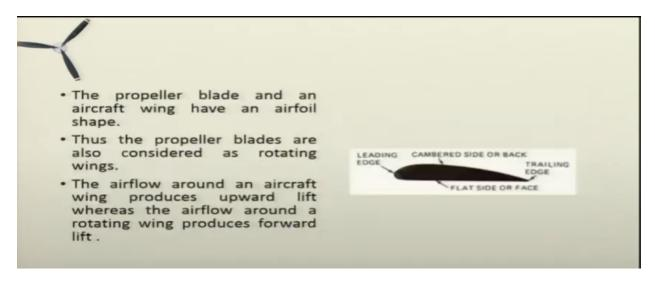
The propeller blade and an aircraft wing have an airfoil shape. Just like the wings of an aircraft, the wings have an airfoil shape; similarly the blades of the propeller also have an aerofoil shape. You can see in the
