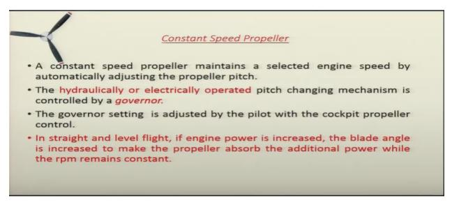
One of the most popular. Propeller used on the aircrafts, on reciprocating engine aircrafts is a constant speed propeller. A constant speed propeller maintains a selected engine speed, by automatically adjusting the propeller pitch. So, this type of propeller, the constant speed propeller, will automatically adjust the
