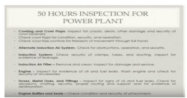
In the 50 hours of operation to sum up there are inspections or cowlings and cowl flaps, alternate induction air system, induction air filter, engine in general hoses, metal lines, and fittings, engine baffles and seals. Refer Slide Time (26:57)
