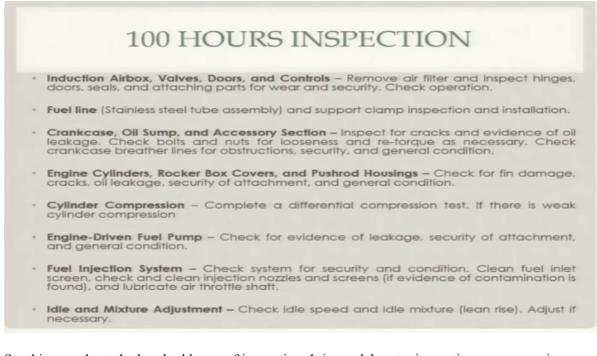
So, this was about the hundred hours of inspection. It is an elaborate inspection you see various areas involved induction air box, walls, doors and controls, fuel line, crankcase, oil sump, and accessory section engine cylinders, rocker box, covers and push rod housings, cylinder compression check, engine driven fuel pump inspection, fuel injection system inspection, idle and mixture adjustment,
