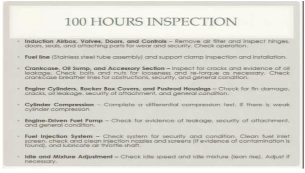
Next inspection is hundred hours of inspection 100 hours of operation. After 100 hours of operation what are the inspections we carried out on the engine. The first area is the induction air box, walls doors and controls. In this we need to remove the air filter and inspect hinges, doors, seals and
