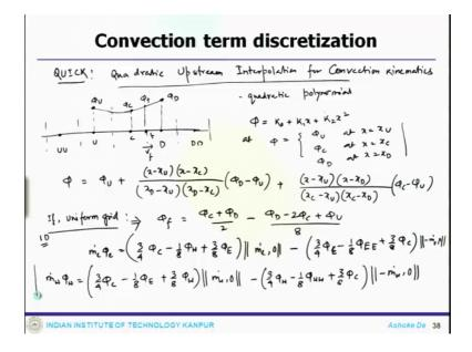
Now in that similar direction one can device another scheme which will call the quick; quick is quadratic upstream interpolation for convection kinematics. So, that is what the quick transfer. So, again if you look at a stencil like that where this is the cell then you have it is the downstream of that it is upstream of that and then this is further upstream this is DD and at the cell phase you can say the v f in this direction and this is the phase value.
