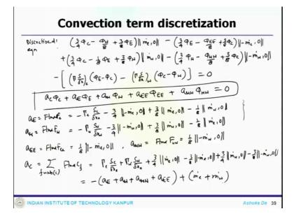
Now, once you do that the discretized terms would look like 3 by 4 phi C minus phi W by 8 plus 3 by 8 phi E that is the first term multiplied with m dot e 0 minus 3 by 4 phi E minus phi EE by 8 plus 3 by 8 phi C multiplied with minus m dot e 0 plus 3 by 4 phi C minus 1 by 8 phi E plus 3 by 8 phi W multiplies with m dot w 0 minus phi W W by 8
