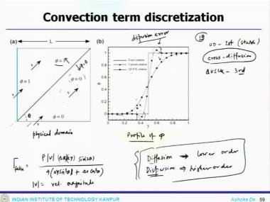
Now, if you look at both the discretized equation, there used for pure advection problem. So, the physical domain one can look at so this is the let us say the physical domain which is shown here, this is the physical domain ok. And this side is the profile of phi along the vertical centre line of the domain for pure advection problem. This is along central line in the y-directions.
