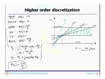
Now, for downwind scheme psi r f equals to 2, and then we see this we can see these things in the psi r f diagram here, which nicely shows the this is the region where all the monotonicity preserving scheme can be found in these particular shaded region. And this is the psi r diagram for higher order scheme and TVD monotonicity preserving scheme.
