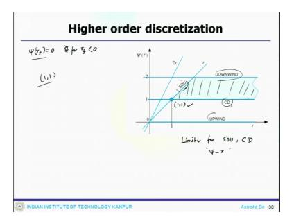
This is the diagram, so which shows the limiters for second order upwind and CD in this psi r diagram. So, one can see that psi if from these diagram you can notice if psi r f equal 0 for r f less than 0. So, r f less than 0, psi r f is 0, the second order accuracy is actually lost at extrema of the solution.
