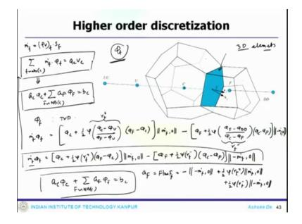
So, what you get essentially combining that to you get the discretized form as a c phi c plus summation of a F phi F equals to b c, where your a F is the flux F f which is minus m dot f 0 plus half psi r f plus m dot f 0 plus half psi r f minus minus m dot f 0.
