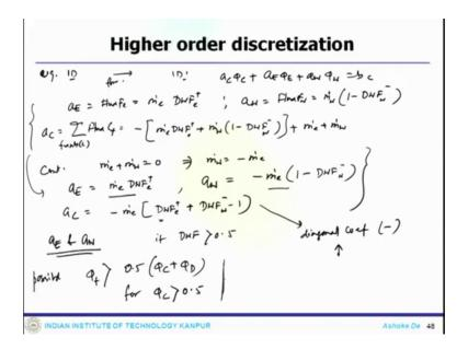
For example 1 D example, now without loss of generality if you assume this is the positive flow direction then the 1 D system would become a C phi C plus a E phi E plus a W phi W equals to b C, where your a E is flux F e which is m dot e DWF plus e, then your a W is flux F w, which is m dot w 1 minus DWF minus F w and a c is summation over faces. So, which is m dot e DWF plus e plus m dot w 1 minus DWF minus w plus m dot e plus m dot w.
