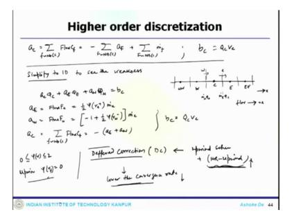
Now, a c would be summation of F nbc which is flux C f, minus F NB C a F plus F NB C m dot f and b c is Q c V c. Now to see the weakness in this formulation so, what one can do, we can this is a multidimensional discretised system, now to see the weakness one can actually simplify to problem to a 1 dimensional system.
